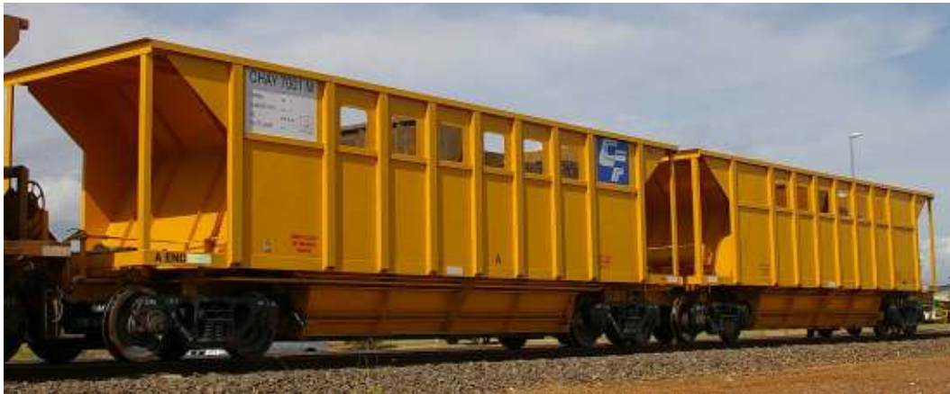
(Note: CHBY 7075 has end deck roof lowered for trials)
